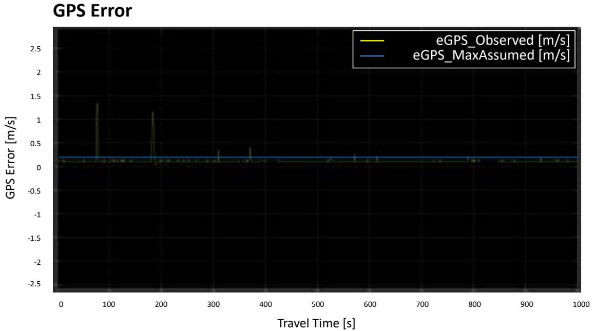
Figure 5.9.: Vehicle Speed Estimation Function: Environment Assumption Monitor for the GPS Data Error during the *Dynamic Driving* Scenario.
